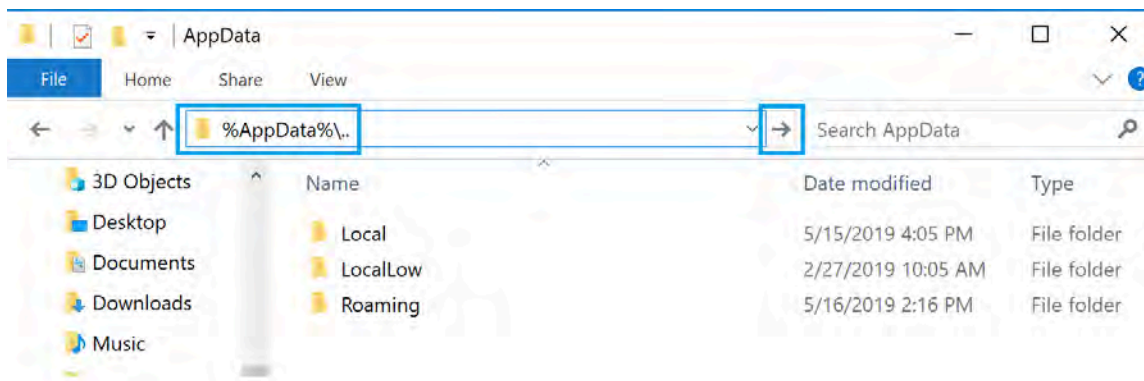
Figure 1.40. Using the %AppData%\.. shortcut in Windows Explorer to access the hidden folder.
