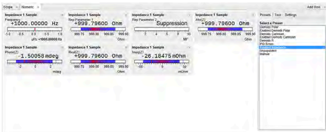
Figure 3.3. Numerical tab displaying measured impedance and circuit representation parameters
