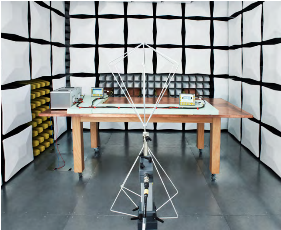
Test setup for component testing in line with MIL-STD-461 and RTCA DO-160 in a compact anechoic chamber.
