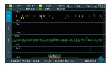
The data logger of the R&S°Scope Rider is used for long-term monitoring of measurement values.
